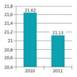
In 2011, water losses were reduced from 21.62% to 21.13%, which is a favourable result given the significant drop in water production. Reductions in water losses are also supported by preventive checks of the water supply network. In 2011, 2,817 km of the water supply network was subjected to checks, revealing 337 hidden water leaks. It will be very difficult to cut the percentage of losses even more without carrying out replacements in the water supply network at the recommended rate.
